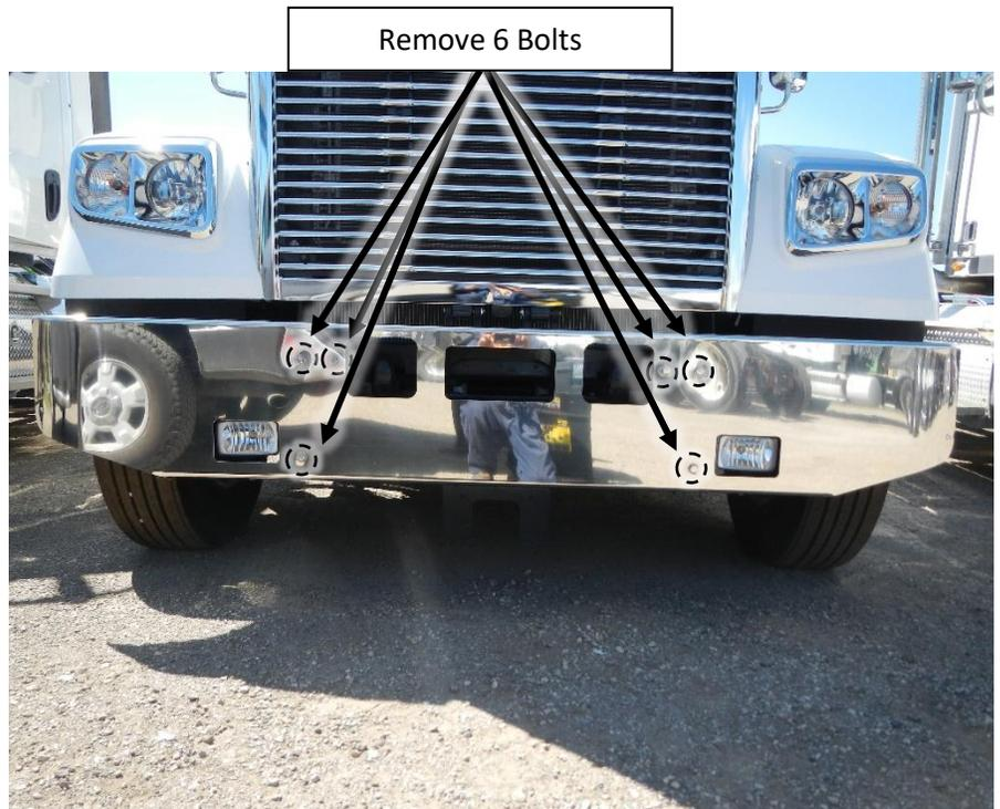
Figure 3 – OEM Bumper Removal Front View
