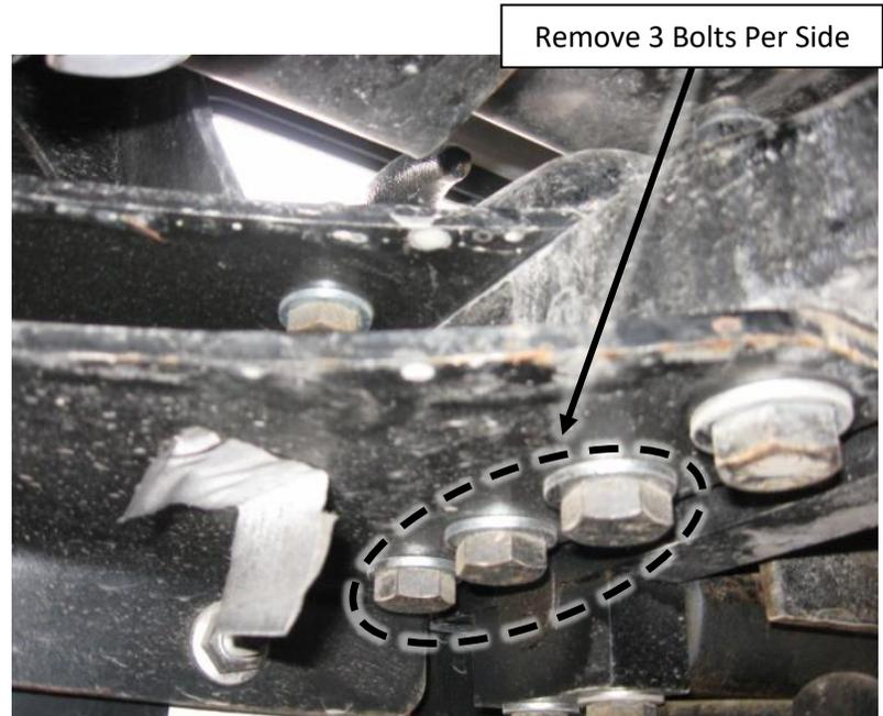
Figure 4 – Tow Hook Removal (Driver Side Shown)
