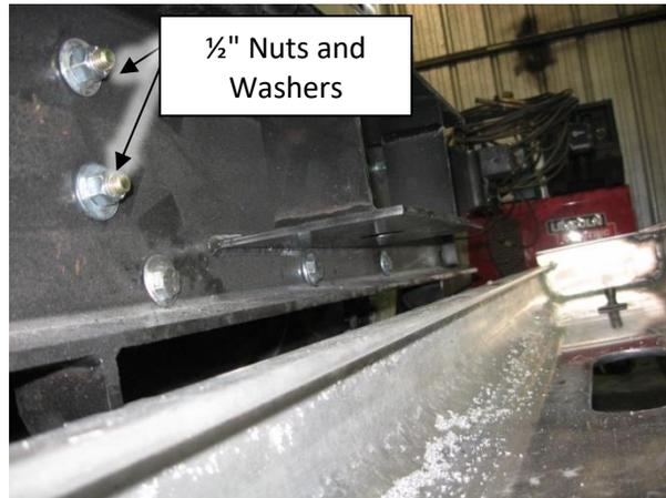
**Figure 8 – HERD Bracket Installation**
