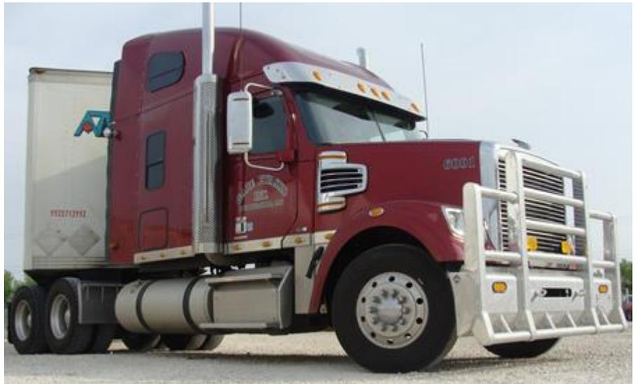
**Figure 10 – Herd Truck Guard Installed**
