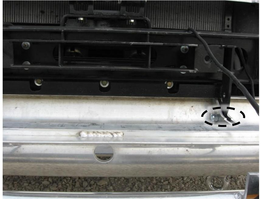
**Figure 9 – View of Bracket Hinge (Driver Side Shown)**
