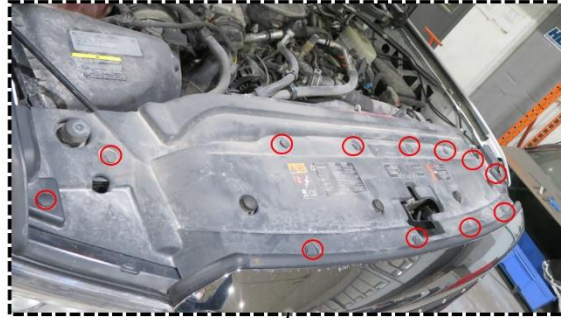
Figure 1a: Remove engine cover
