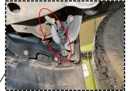
Figure 1c: Remove bottom mounting bar (passenger side shown)
