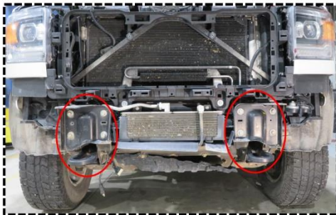
Figure 1e: Remove OEM tow loop
