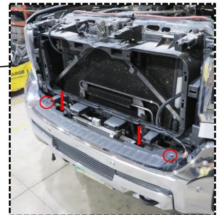
Figure 1d: Remove front bumper
