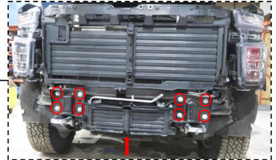
Figure 2e: Remove bumper
