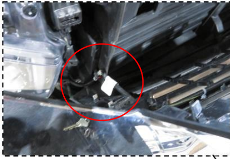
Figure 2b: Unplug the camera connector
