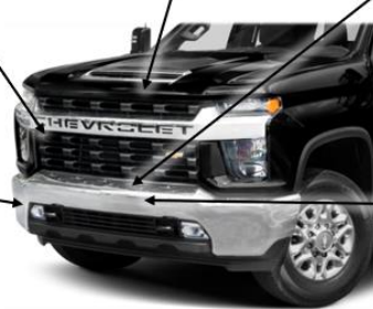
Figure 2a: Remove front grille
