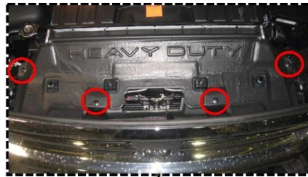
Figure 1a: Remove engine cover
