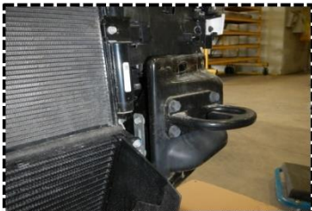
Figure 1e: Remove OEM tow loop
