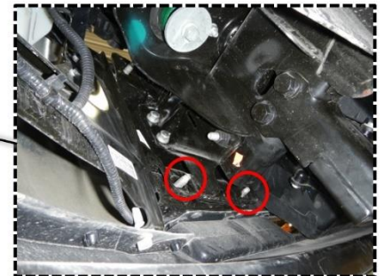
Figure 1d: Remove front bumper (view from under)
