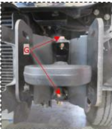
Figure 2f: Submounts installation (driver side front view)
