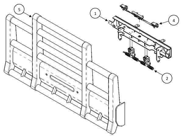
Figure 2 – Slam Latch Latching System
