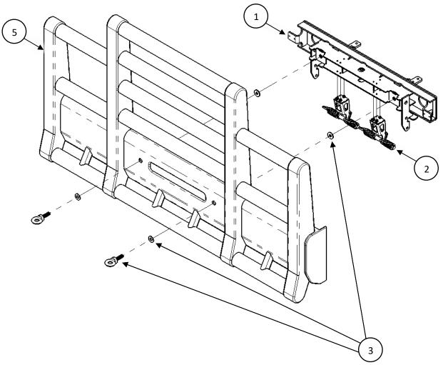
Figure 1 – Captive Eye Bolt Latching System
