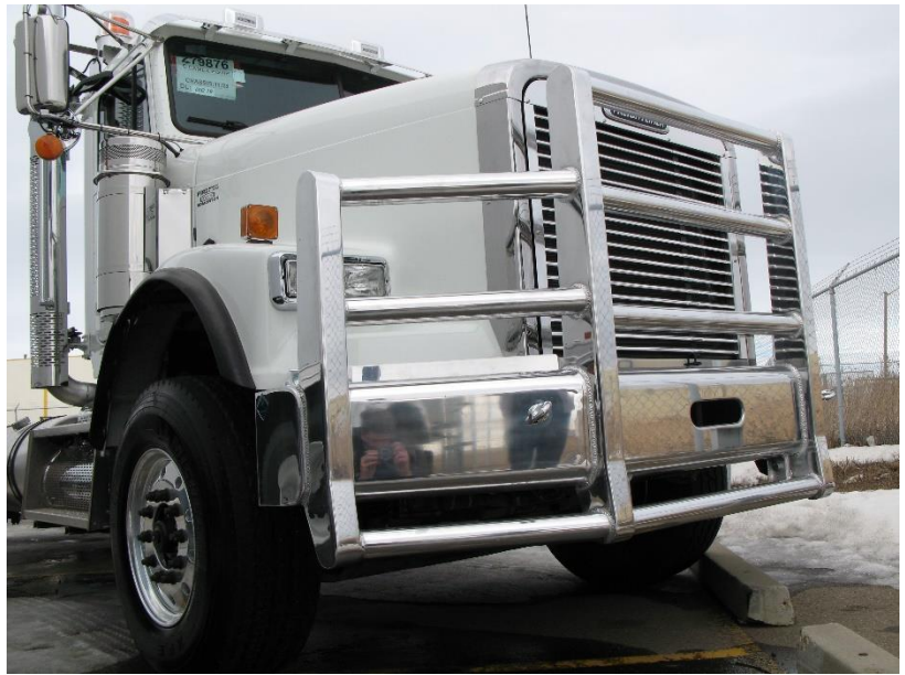
Figure 8 – Herd Truck Guard Installed
