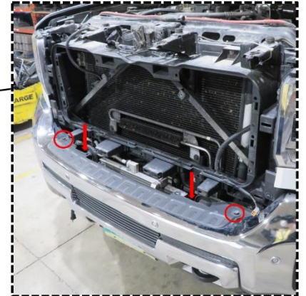
Figure 1d: Remove front bumper
