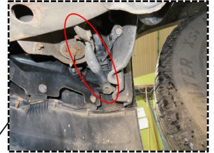
Figure 1c: Remove bottom mounting bar (passenger side shown)
