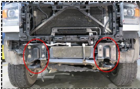
Figure 1e: Remove OEM tow loop
