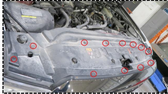
Figure 1a: Remove engine cover
