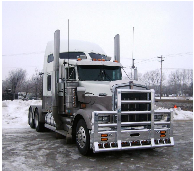
Figure 8 – Herd Truck Guard Installed
