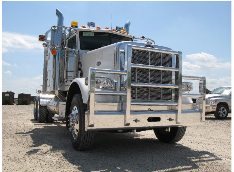
Figure 10 – Herd Truck Guard Installed
