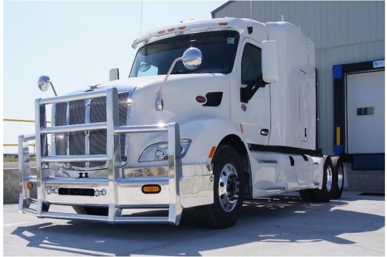
**Figure 12 – Herd Truck Guard Installed**
