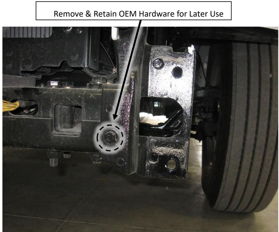
**Figure 4** – OEM Bolt Removal (Drivers Side Shown)
