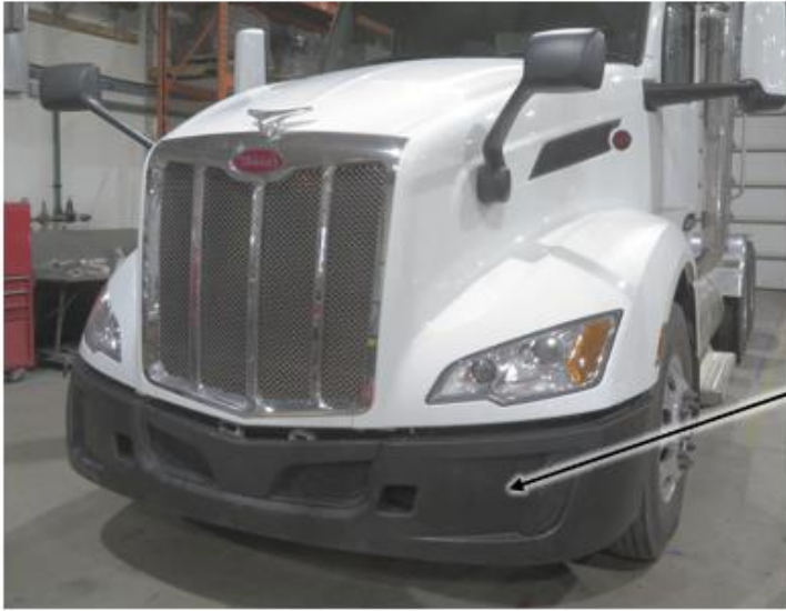
Figure 1: Removing the OEM Front Bumper (Your Truck may not be exactly as shown)
