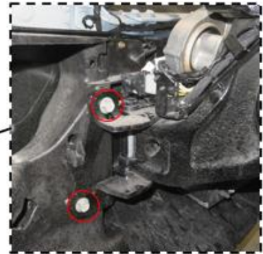
Figure 1a: OEM Front Bumper fasteners (DS shown)
