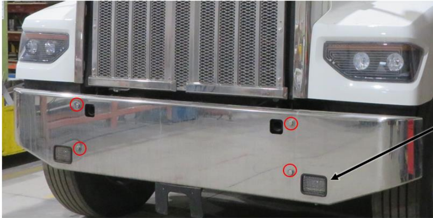
Figure 1b: Remove OEM Front Bumper
