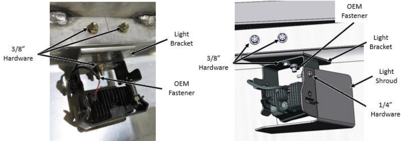
Figure 3a: OEM Lights and HERD Light Bracket on an SFA Truck (DS Shown)
