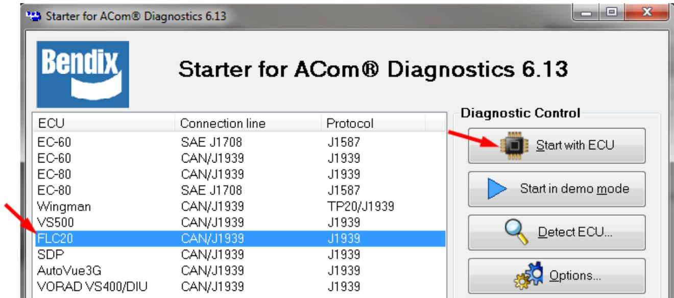
NOTE: When using ACom Diagnostic Software for first time, service technician will be asked to select communication adapter for the Bendix® Fusion™ FLC20™ camera. Technician will need to indicate which communication protocol to use. Once a successful connection has been made, these steps will no longer be necessary.
