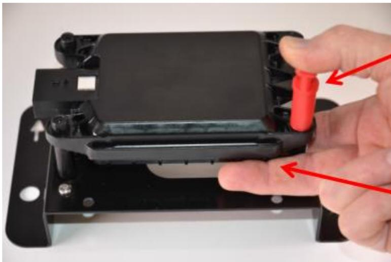
**Insert and hold the release tool on the clip**
