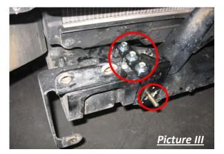
5 Mount Herd bracket to truck, with packers (3) for spacing on the bottom bolts, using Herd supplied bolts ( $\frac{1}{2}$ " x 3<sup>1</sup>/<sub>2</sub>" and  $\frac{1}{2}$ " x 2")
