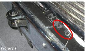
Remove the factory bumper mounting brackets by removing the three (3) bolts & sensor mount (driver side only) from each side of the frame. (Picture II)
