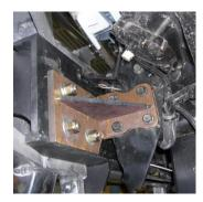
Eyebolts are secured in the channel with a 7/8" rubber washer. If you need to re-install the washer, insert the eyebolt into the hole, and thread a washer onto the back side of the eyebolt, approximately halfway onto the threaded part of the eyebolt.
