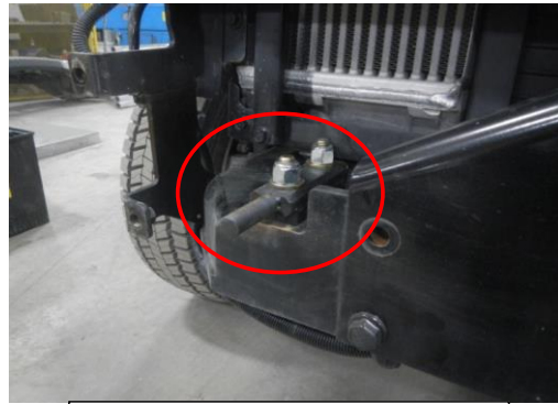
Herd Tow Section mount - installed
