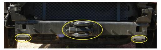
3 Install the HERD Suppiled lower mounts using the OEM Hardware
