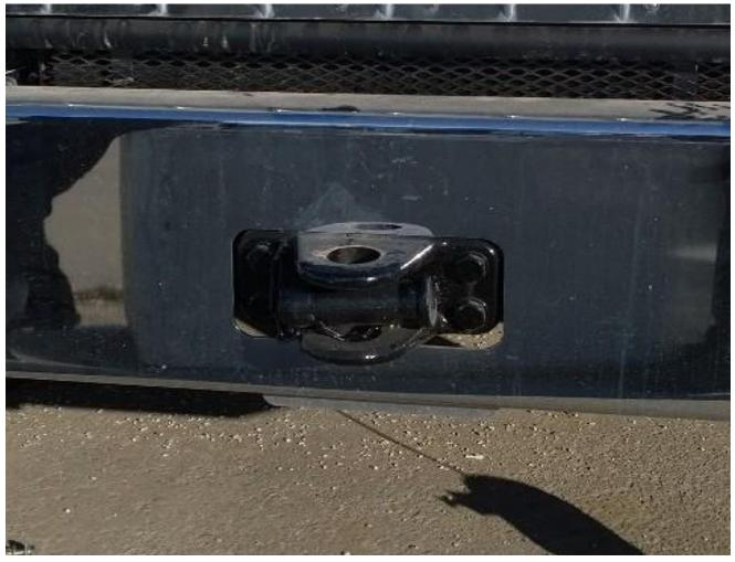
2 Remove lower bumper mounts from the factory tow section on each side, see picture below.
