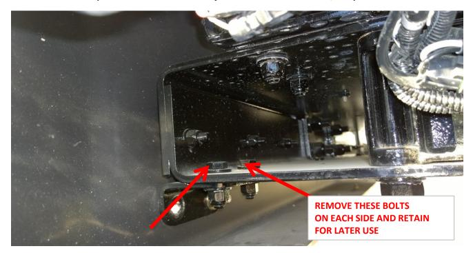
3 Remove the top bumper mounting bolts, see picture below
