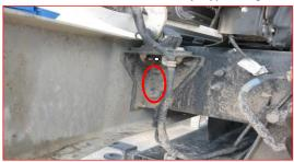
3 Mount Herd sub mounts onto back of bracket (see picture below) and then position these bracket mounts between truck frame rails. Bolt the Herd mounts to the frame rails utilizing the holes exposed when the factory bolts were removed.
