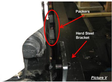
7 Attach bullbar to bracket using Herd supplied hinge bolts
