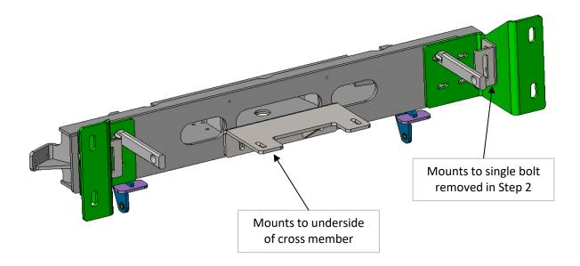
4 Attach bullbar to bracket using Herd supplied hinge bolts, Pictures below locates brackets to truck.
