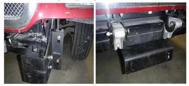
**Note:** \* For DFLT & Defender models only: To install the hinge bolts, the bumper must be in the open (down) position to allow the bottom lip to go under and around the steel hinge.
