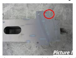
Locate the top two holes of the six that are near the tow box (on the Herd steel bracket) and mark the crossmember behind those holes for drilling (Picture II)
