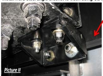
Install Herd steel bracket to truck using OE hardware (do not tighten at this point of installation) and install packers using Herd supplied bolts (3/4" x 3"). (Picture |||)
