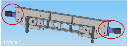
3 Install Herd steel bracket onto truck using OE hardware on centre 6 holes only (Picture II)
