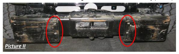
Install Impact Plates on the back side on the outside top two mounting holes using the bolts from
