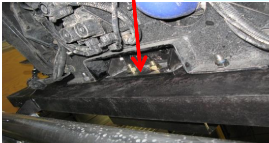
Lower loose bracket bolts to the back of the steel bracket & to this bolt on the frame
