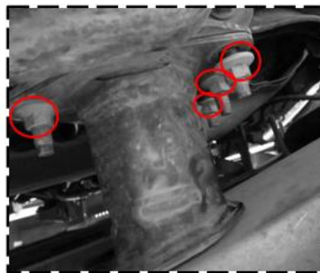
Figure 1d: Frame Rail Fasteners Removal (Driver Side Shown)
