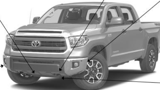
Figure 1d: Frame Rail Fasteners Removal (Driver Side Shown)
