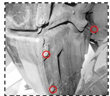
Figure 1c: Fender Liner Removal (Driver Side Shown)
