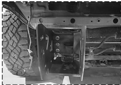
Figure 2a: Submount Installation
