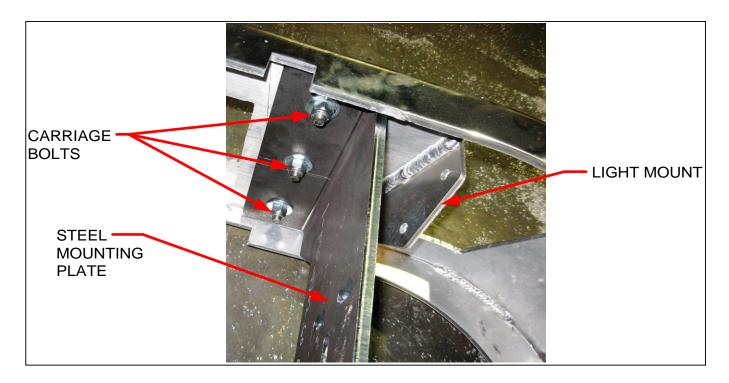
4 Install Herd aluminum bumper to steel mounting plates with supplied carriage bolts, as shown above.
