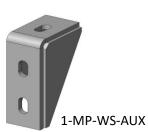
The loose part (1-MP-WS-AUX, see above) will go underneath the frame member, and bolt to the Herd bracket using the supplied hardware. The frame rail should be sandwiched between this loose piece and the angle bracket welded to the back of the Herd bracket.
