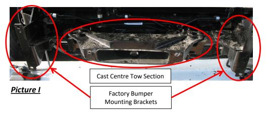
Install Herd steel bracket to truck using supplied hardware (thin shims have been provide and may be required at the outside most mounting holes to ensure the bar sits square on the truck - see Picture II)
