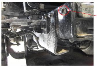
REMOVE AND REPLACE FIRST BOLT EACH SIDE WITH 2-1-2" BOLTS, FLAT WASHERS, AND LOCK NUTS
