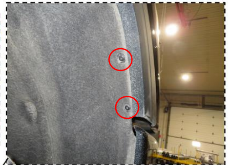
Figure 1c: Remove fender liner screws (passenger side shown)
