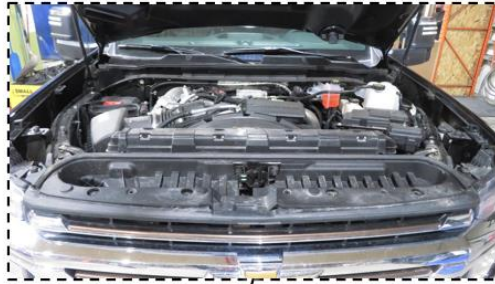
Figure 1b: Remove radiator cover
