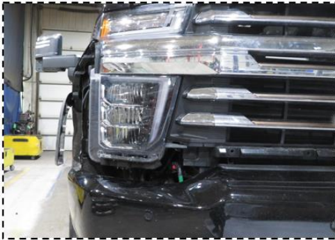
Figure 1e: Remove valance (passenger side shown)
