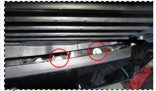
Figure 2d: Remove bumper fasteners (driver side shown)
