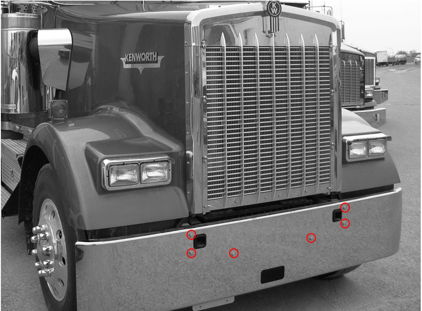
Figure 1: Removing the OEM Front Bumper (Your Truck may not be exactly as shown)
