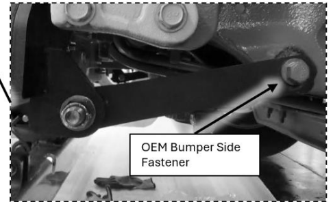
Figure 2d: Driver Side Submount Installation (Side View Shown)
